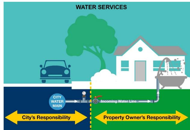
drinking water, any service lines identified as lead must be replaced within 10 years.
